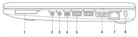
1 ExpressCard slot – Supports one ExpressCard. The computer ships with a plastic blank installed in the slot.
