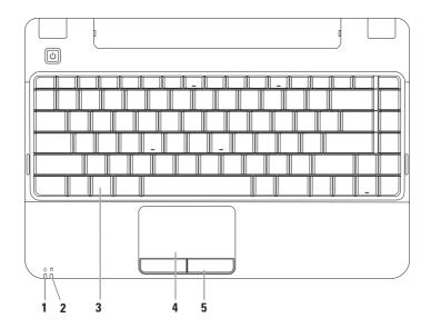
1 Power/Battery indicator light – The light indicates the following states when powered using an AC adapter or a battery.
