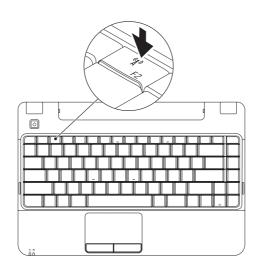
1. Press the <F2> key or press the <sup>6</sup>A³ key on the keyboard to enable or disable wireless. The wireless enable or disable dialog box will appear on your screen.
